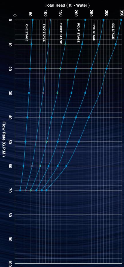
1 STAGE = 1.5 HP 2 STAGE = 3 HP 3 STAGE = 3 HP 4 STAGE = 5 HP 5 STAGE = 5 HP 6 STAGE = 7.5 HP
