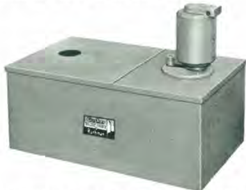
The split lid design, shown here on the Model T-50, is furnished as standard on all models except CB styles. On models T-80 and larger, the reservoir is angled to permit chip removal with a shovel or hoe.
