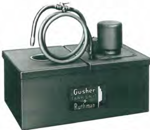
Gusher Model T-10M, shown with optional hose, nozzle and valve assembly, typifies the standard tank unit design. Swivel casters are also available optionally on models thru T-80F for added portability.
