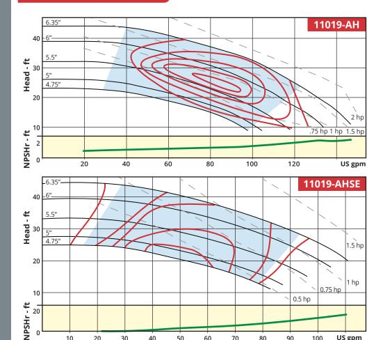
\*11019-AH and 11019-AHSE 1750 RPM pumps are available in 1 hp, 1.5 hp and 2 hp models. Other hp shown for reference only.
