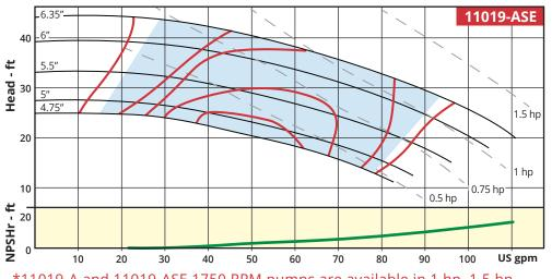
\*11019-A and 11019-ASE 1750 RPM pumps are available in 1 hp, 1.5 hp and 2 hp models. Other hp shown for reference only.
