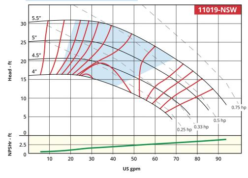
\*11019-NS-W 1750 RPM pump is available in 1 hp model only. Other hp shown for reference only.
